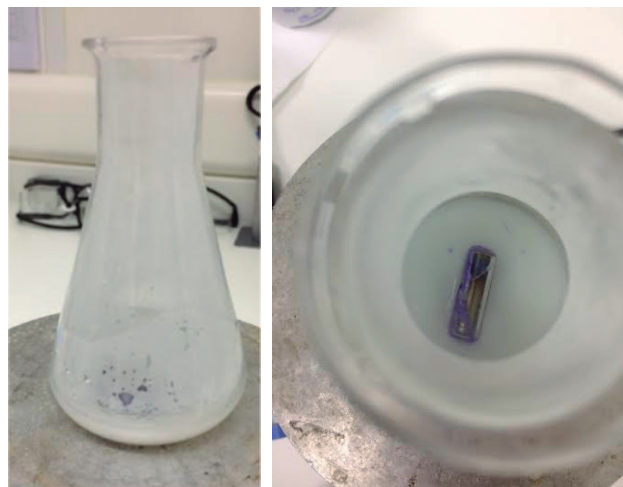
Figure 1 – Appearance of the nanoparticle emulsion before the addition of the alcoholic plant extract
